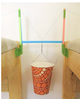
Attach the load tester (cup) to the bridge deck (the blue straw here) as you did before.
