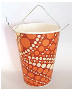
Make a load tester by bending a large paperclip into a V-shape and poking the ends into a paper cup, on opposite sides just below the rim.
