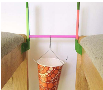
Attach the load tester (paper cup) to the bridge deck (the pink straw here) by using a second large paperclip.
