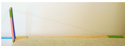
Attach each end of the cable to a paperclip and tape the paperclip to the furniture, as shown here (for only the right side of the bridge), so that the cable is tight.
